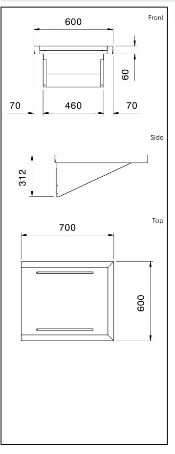
Handling System for Hood type Dishwasher Service Shelf, 700mm (entry level HT)
